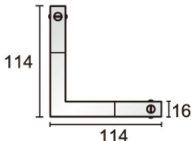
After inserting into the track, rotate the lock counterclockwise to fix the conduction and load bearing fixation!
